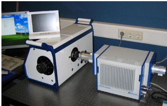
Figure 5. Framing Camera and Streak Camera layout for test.
