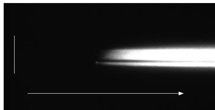
Fig. 3 Streak Record, 100 ns/mm writing speed, ~ 2 usec total time window.
