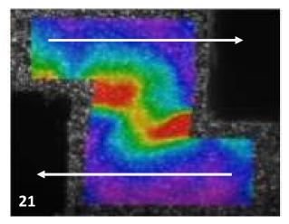
In an adiabatic shear test such as this, the strain localises along precise shear bands. This occurs due to high-strain rate loading giving rise to localised heat concentrations which do not have time to conduct in the bulk material. This high temperature 'band' deforms far more readily than the cooler bulk material. In a slower, more static test the strain field would be less localised, due to these isothermal conditions.
