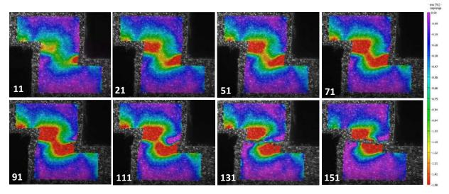
The imaging results were analysed using Correlated Solutions Vic-2D DIC software. The above analysis show exx lagrange strain (strain in the same direction of motion) for the same images shown previously.
