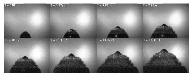
Using the static image to calibrate the dynamic sequence the tip velocities in images 2 – 8 could be measured using the SIM software measurement function.
