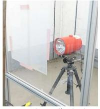
a 30ms time window, but later test capture windows were between 5µs and 12µs. Illumination was provided by an SI-AD500 flash lamp placed behind the detonator to provide a shadowgraph image through a diffuser. Flash lamp duration was 2ms with a rise time 80µs. Both cameras and flash lamp were protected using 5mm thick Perspex.
