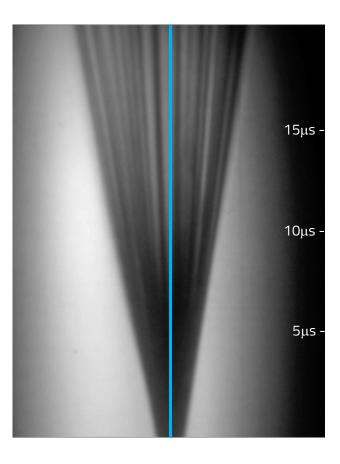
From this the case diameter expansion velocity was calculated to be approx. 2,200m/s.
